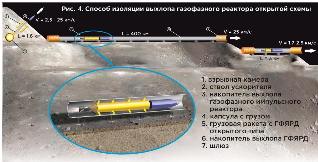
Fig. 4. Non-explosive transport technology - launching cargo ships with an open circuit gas-phase nuclear rocket engine. A method for isolating and storing exhaust from an open-circuit gas-phase reactor.
